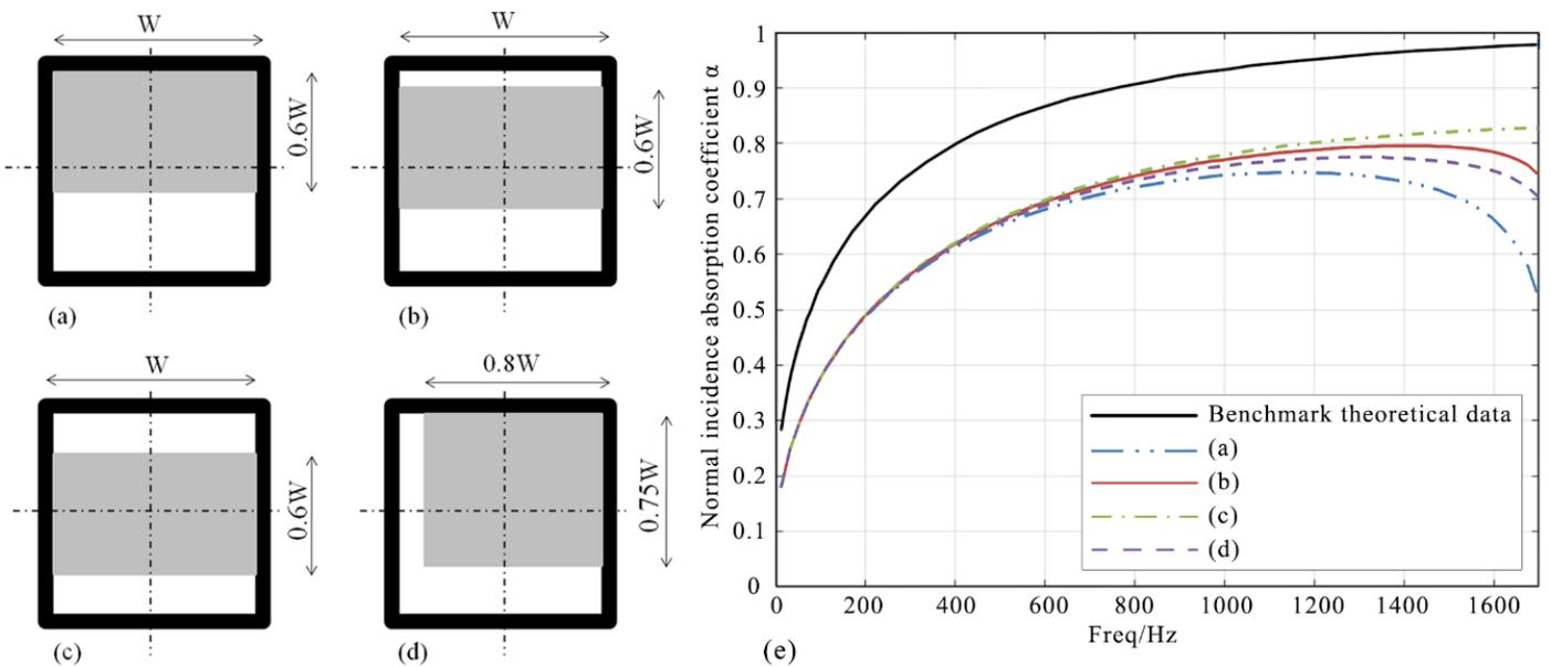
Figure 2: Effects of sample positions ((a), (b), (c)) in the SWT and shape (d) on sound absorption coefficient (e) of DIB. (Note: the areas of (a), (b), (c), and (d) are equal)
