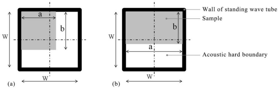
Figure 1: Schematic diagrams of the relation of cross section size between porous material sample and the square SWT
