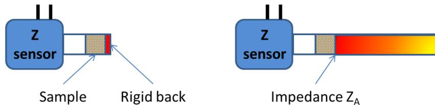
Figure 1: Measurement procedure with two acoustic loads
